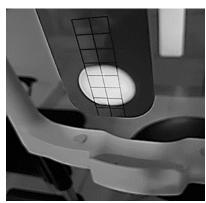
Once the light beam focus is finely adjusted, remove the ABF Plate from the forehead strap of the slit lamp and proceed with laser treatments.
